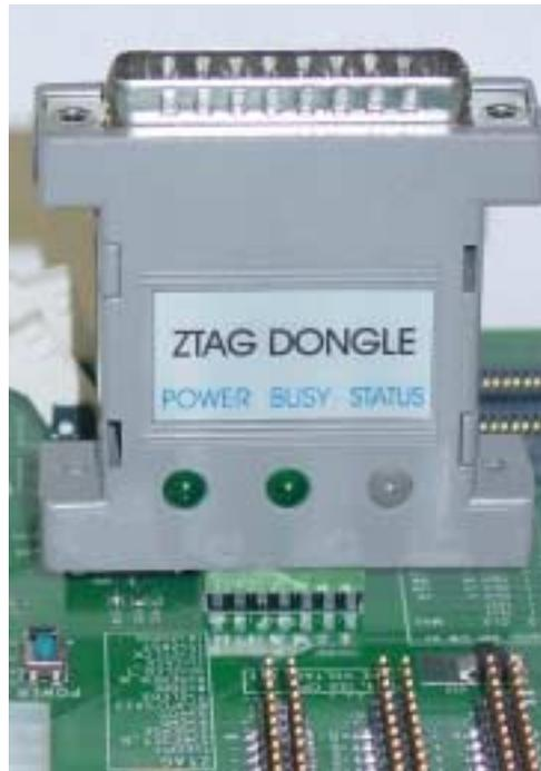
*Figure 1.3 Z-tag Dongle Connected to the IDS Board*
