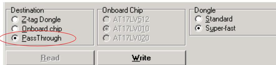
Figure A.6 Verify the Z-tag Dongle is Enabled
