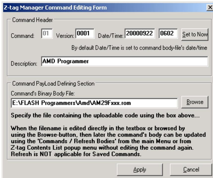
Figure A.3 Adding AMD Flash Programmer Code To The Upload & Execute Command
